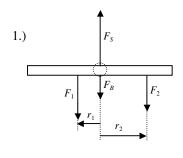
$$F_B = 40 \text{ N}, F_1 = 500 \text{ N}, \text{ and } F_2 = 350 \text{ N}$$
