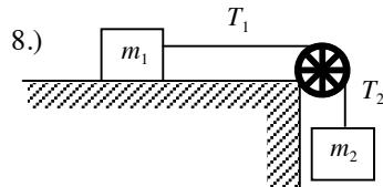
$m_1 = 2.0 \text{ kg}$ ,  $m_2 = 1.5 \text{ kg}$  and the pulley is hollow cylinder  $M = 1.0 \text{ kg}$ ,  $R = 0.15 \text{ m}$
