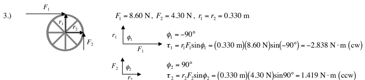
$$\tau_{net} = \tau_1 + \tau_2 = -2.838 \text{ N} \cdot \text{m} + 1.419 \text{ N} \cdot \text{m} = -1.419 \text{ N} \cdot \text{m} (\text{cw})$$
