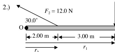
$$\tau_1 = r_1 F_1 \sin \phi_1 = (5.00 \text{ m})(8.00 \text{ N})\sin(-90^\circ) = -40.0 \text{ N} \cdot \text{m} (\text{cw})$$
