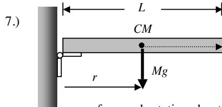
a.) rotation results from the torque due to the weight of the rod
