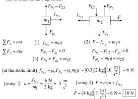
Example 12:  $m_1 = 2 \text{ kg}, m_2 = 4 \text{ kg}, \text{ between blocks } \mu_s = 0.3 \text{ and } \mu_k = 0.2$  frictionless table
