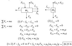
Example 10b:  $m_1 = 5.4 \text{ kg}, m_2 = 2.7 \text{ kg}, \mu_k = 0.25$ moving with constant speed (a = 0), F = ?
