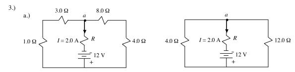
The equivalent resistance for the entire circuit is:  $R_{eq} = \frac{V_{12V}}{I} = \frac{12 \text{ V}}{2 \text{ A}} = 6 \Omega$
