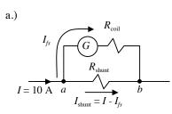
Ammeter reading 10 A full scale.
