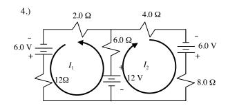
a.) Using Loop Method (Mesh Currents):
