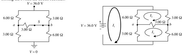
The circuit is like the bridge circuit on HO 36 with nothing in parallel or series. Using Loop Method:
