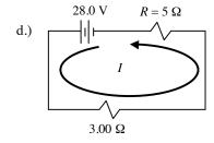
Applying Kirchhoff's Loop rule:  $V_{28V} = V_R + V_{3\Omega} = IR + IR_{3\Omega}$
