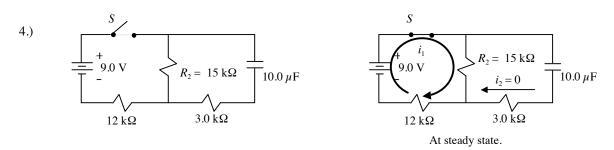
a.) At steady state the capacitor is fully charged and current has decayed to zero.
