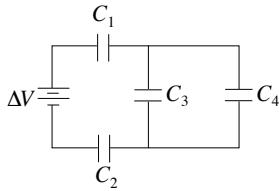
In the above circuit  $C_1 = 40 \mu\text{F}$ ,  $C_2 = 60 \mu\text{F}$ ,  $C_3 = 50 \mu\text{F}$ ,  $C_4 = 70 \mu\text{F}$ , and the potential difference  $\Delta V = 120 \text{ V}$ .
