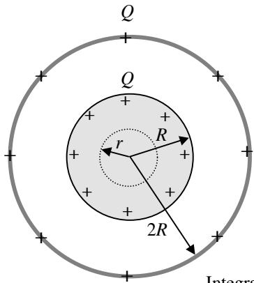
$$V_a - V_b = - \int_b^a \vec{E} \cdot d\vec{r} \quad \text{and get } E \text{ using Gauss's Law.}$$
