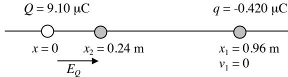
$$k \frac{Qq}{x_1} = \frac{1}{2} mv_2^2 + k \frac{Qq}{x_2} \quad (K_1 = 0 \text{ since } v_1 = 0) \quad \text{so} \quad \frac{1}{2} mv_2^2 = k \frac{Qq}{x_1} - k \frac{Qq}{x_2} = kQq \left( \frac{1}{x_1} - \frac{1}{x_2} \right)$$
