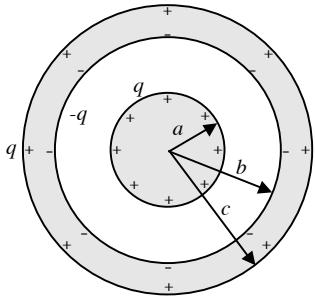
$$V_a - V_b = - \int_b^a \bar{E} \cdot d\bar{r} \quad \text{and get } E \text{ using Gauss's Law.}$$
