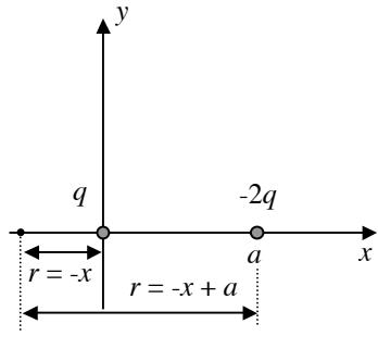
$$V = \sum \frac{kq}{r} = k\left(\frac{q}{-x} + \frac{-2q}{-x+a}\right) = k\left(\frac{-q}{x} + \frac{2q}{x-a}\right) = k\left(\frac{-q(x-a) + 2qx}{x(x-a)}\right)$$
