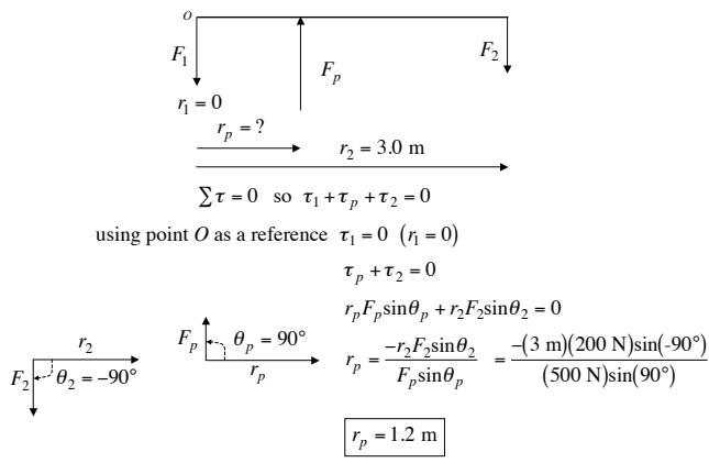
Example 1b:  $\ell = 3.0 \text{ m}$ ,  $F_1 = 300 \text{ N}$ ,  $F_2 = 200 \text{ N}$ ,  $F_p = 500 \text{ N}$
