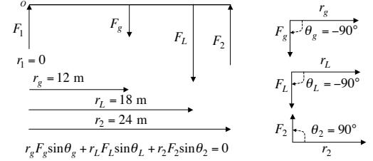
$$F_2 = \frac{-(r_g F_g \sin \theta_g + r_L F_L \sin \theta_L)}{r_2 \sin \theta_2} = \frac{-((12 \text{ m})(900 \text{ N}) \sin(-90^\circ) + (18 \text{ m})(12,000 \text{ N}) \sin(-90^\circ))}{(24 \text{ m}) \sin(90^\circ)}$$
