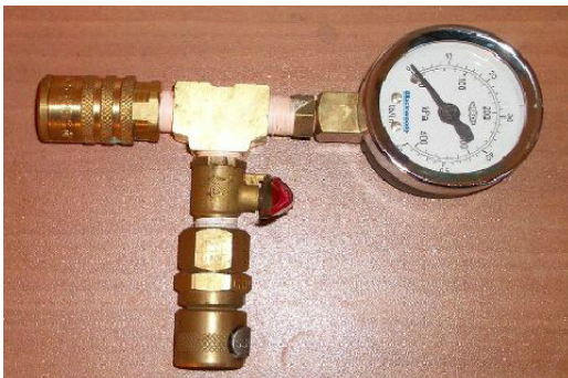
Fig 20.4: Autoclave pressure head
