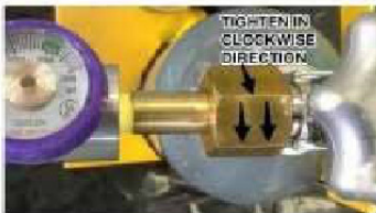
Fig 5.24 Attaching the regulator to the cylinder:
