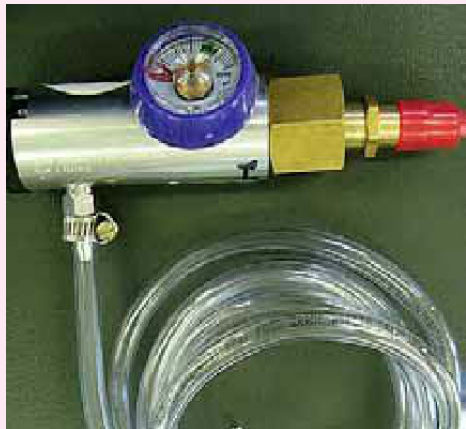
Fig 5.19: 6mm PVC tubing attached to MaxDog gas regulator
