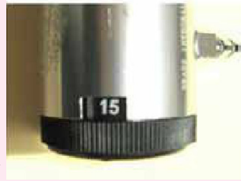
Fig 5.26: Gas flow @ 15l/min
